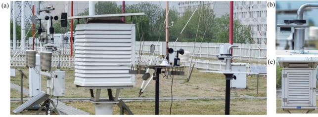
Fig. 4. Photos of the experimental setup: (a) the entire experimental field, (b) and (c) the screen and the aspirated temperature measurement platform, respectively.
