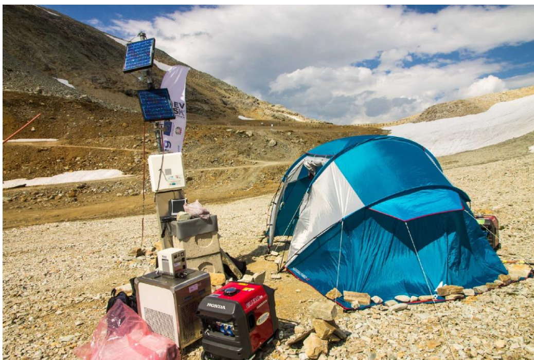
Figure 17, A calibration laboratory at 3000 m of altitude at the Sommeiller pass, for the calibration of permafrost sensors chains.
