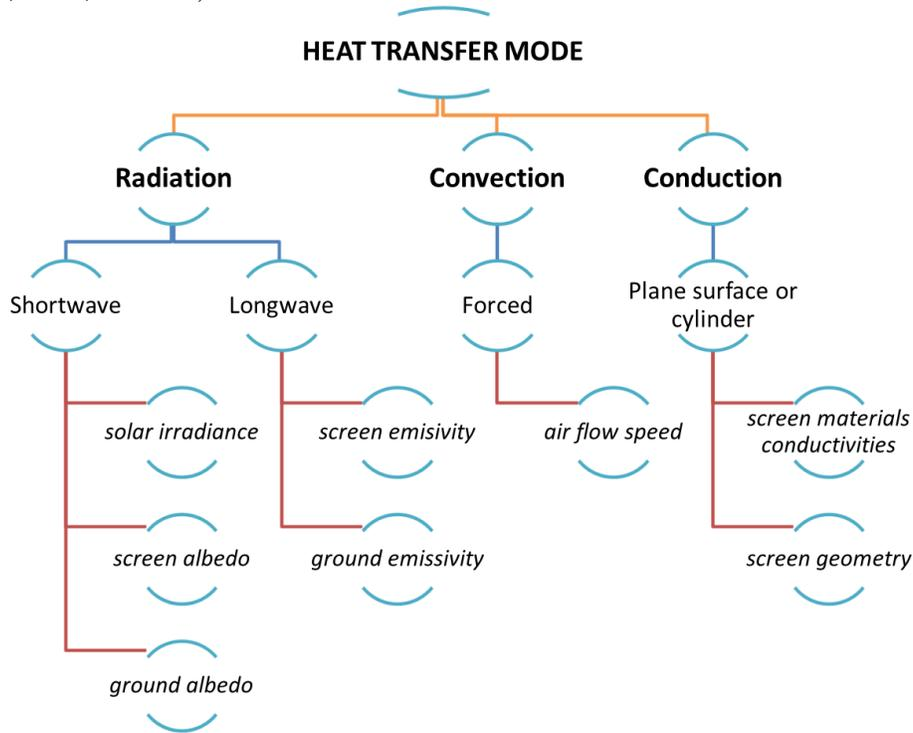
**Figure 2.** Ambient parameters contributing to heat transfer inside a meteorological shelter
