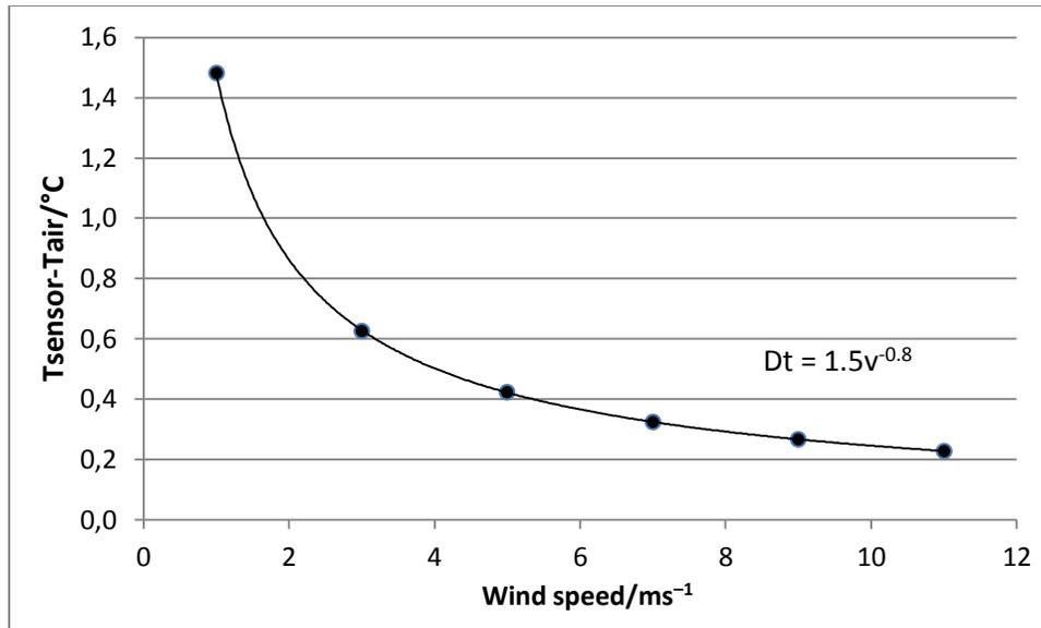
**Figure 6.** Temperature difference of the air inside the shield and surrounding air for different wind speed at maximum solar irradiation ( $1000 \text{ Wm}^{-2}$ ).
