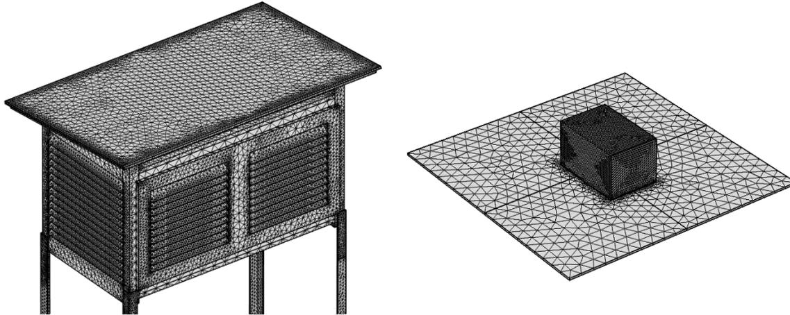
**Figure 3.** Screen and domain mesh.
