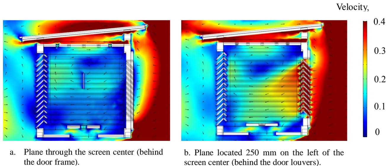
**Figure 4.** Velocity profile inside the shield.
