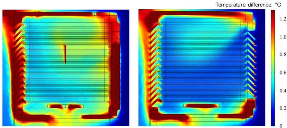
**Figure 5.** Temperature difference of the air inside the shield and surrounding air. Left: the plane cutting through the thermometer center (behind the door frame). Right: the plane located 250 mm to the left of the thermometer (behind the door louvers).
