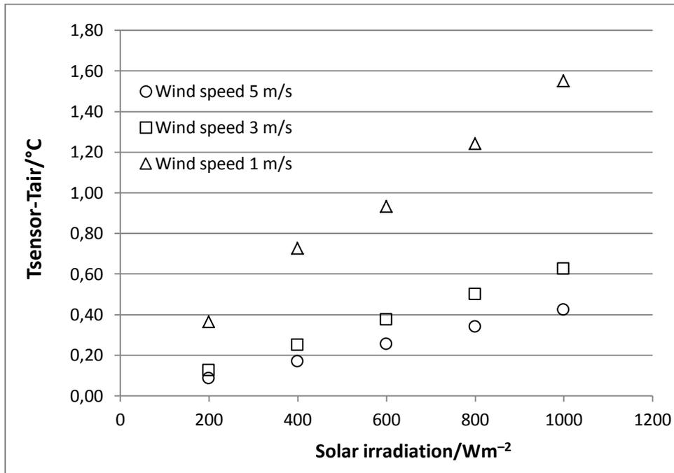
**Figure 7.** Temperature difference of the air inside the shield and surrounding air for different solar irradiances at different wind speeds
