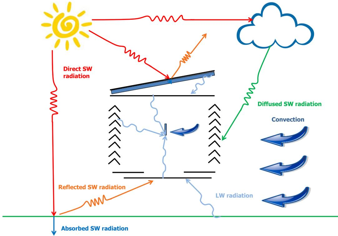
**Figure 1.** Heat transfer modes involved in modeling the measured temperature inside a meteorological screen.
